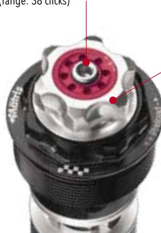
**Preload** unit assembled on axial roller bearings, with reference clicks
