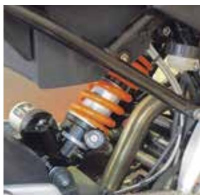
Separate pressurized expansion tank
